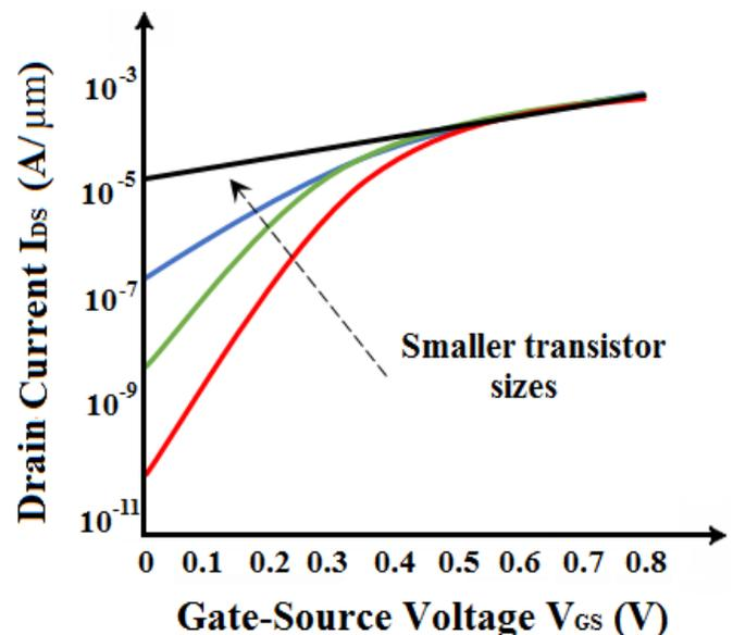
Fig. 1. Gate voltage versus drain current.
